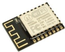
Gambar 5. Modul wifi ESP 12-E
