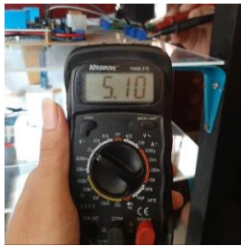
Gambar 10. Tegangan Output Voltage Regulator
